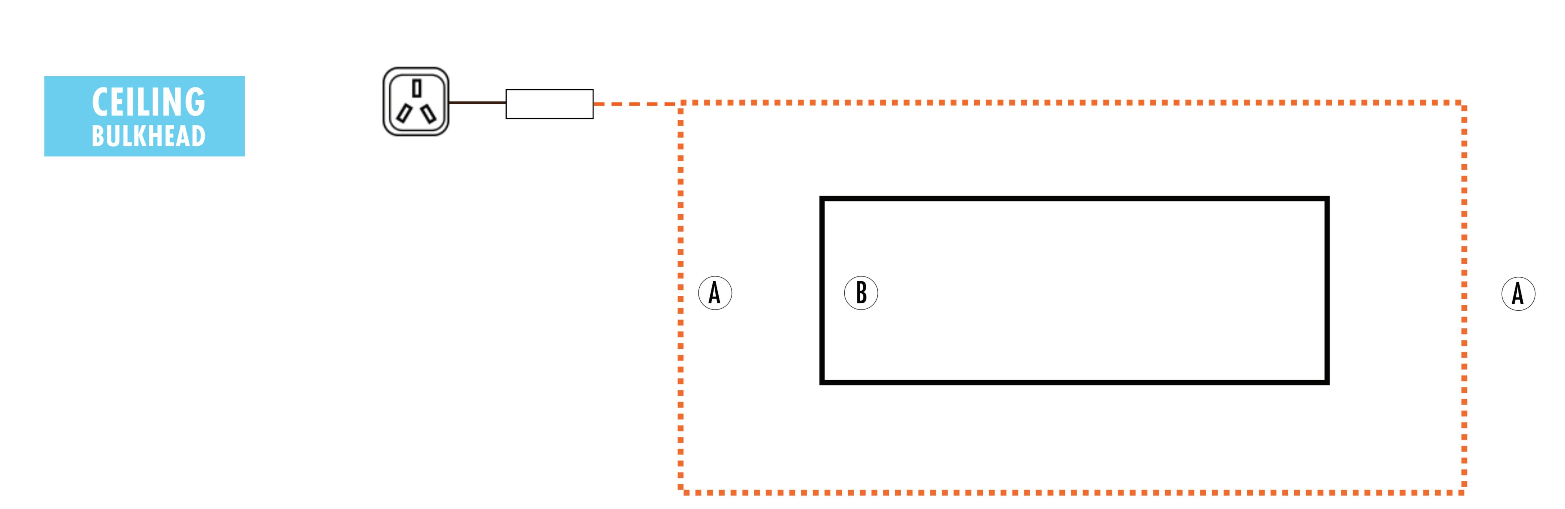
Wrap around bulkhead on the back of the recess, facing inwards.
