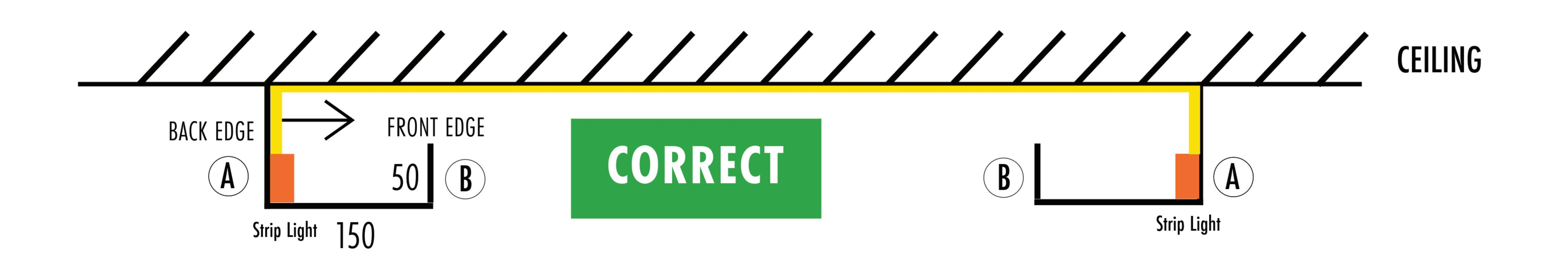
For recess size similar to 150(w) x 50(h). Place strip sideways facing in on back edge (A) of recess
